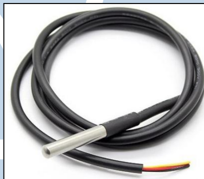
Gambar 2. 9 Sensor Suhu Waterproof DS18B20 (sumber: makerlab-electronics.com)
